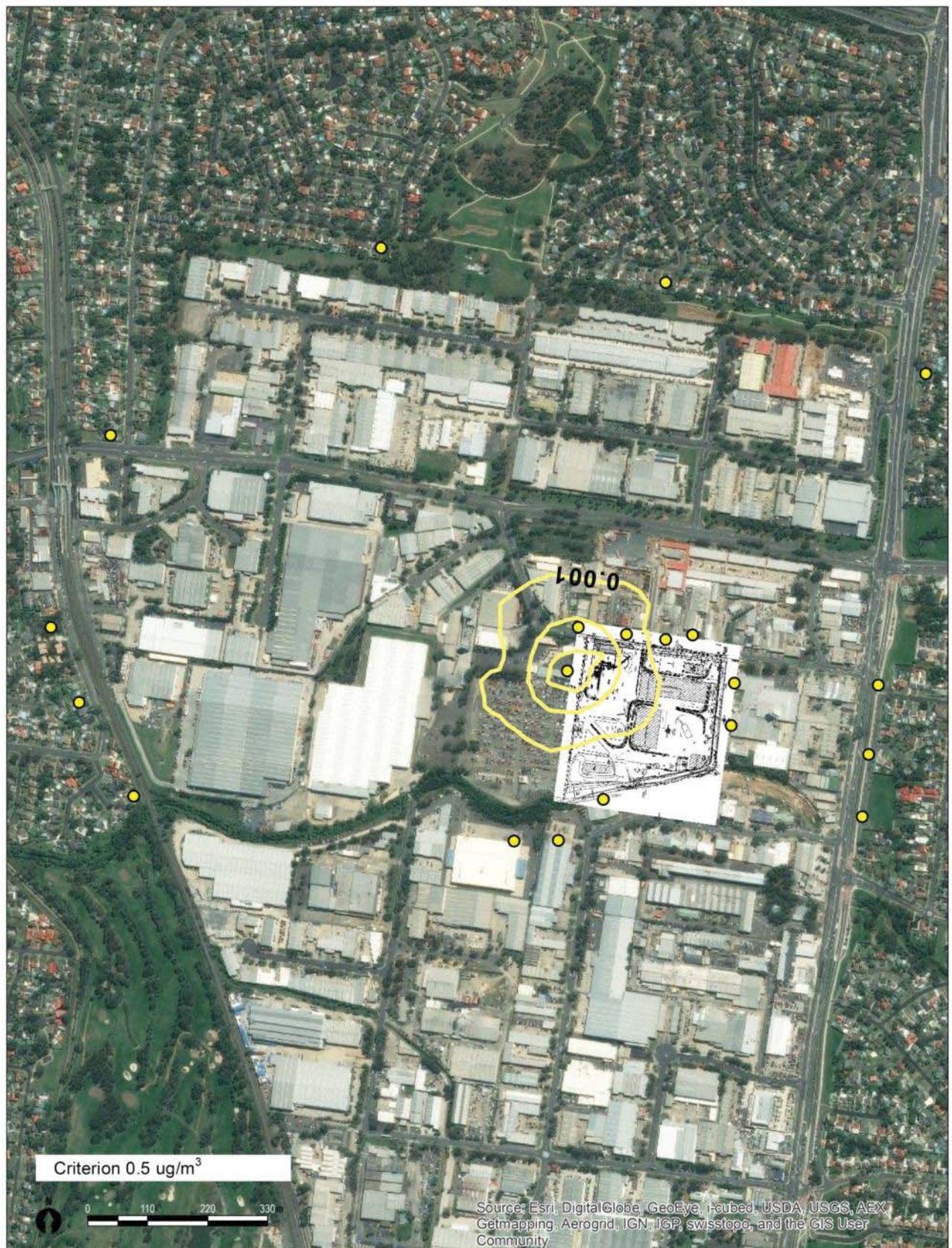
Figure B.6 Maximum predicted (over five years) Site contribution to annual mean lead concentrations (excluding background)
