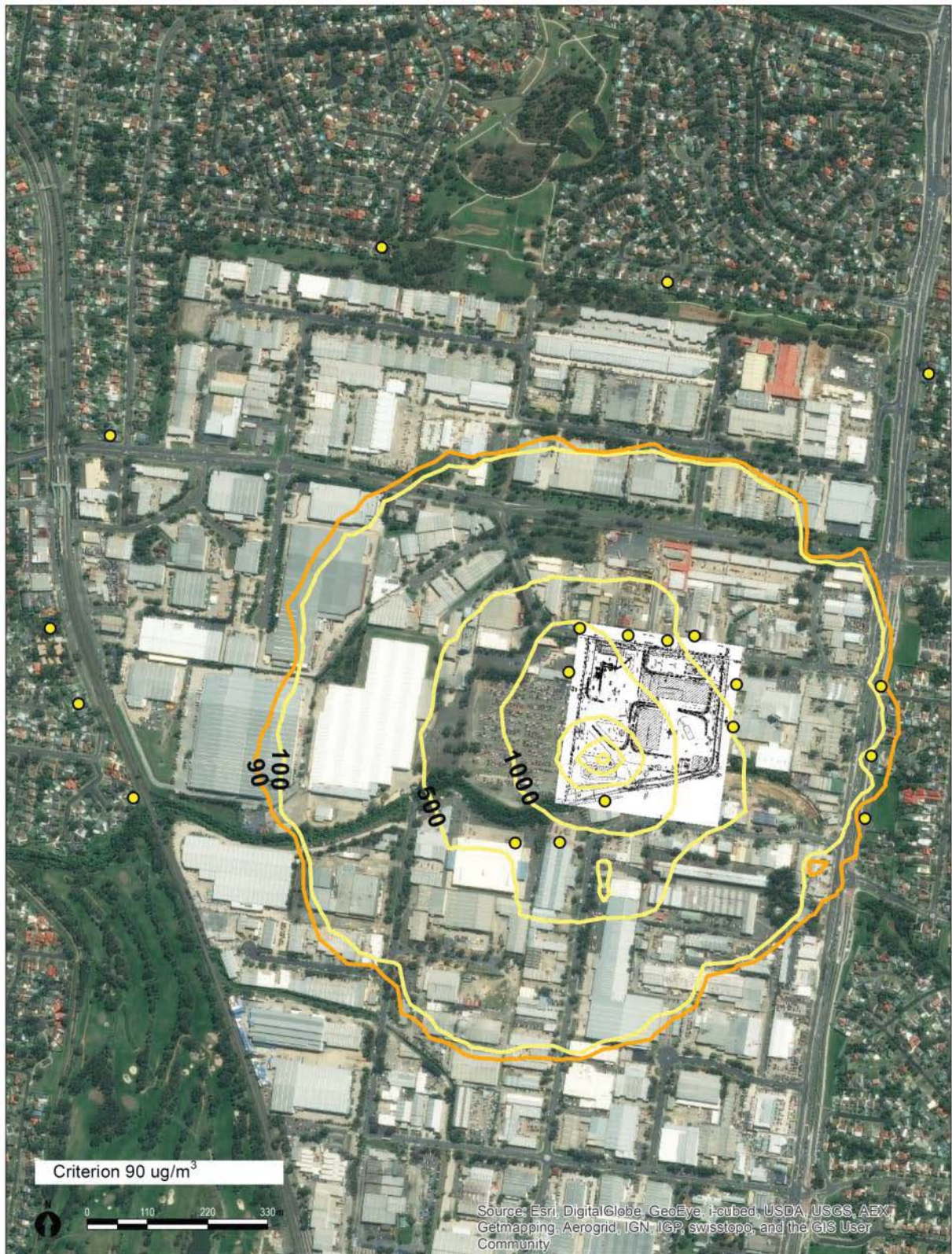
Figure B.16 Maximum (99.9 th percentile) predicted (over five years) Site contribution to hourly iron oxide fumes concentrations (excluding background) with cutting modelled as point sources
