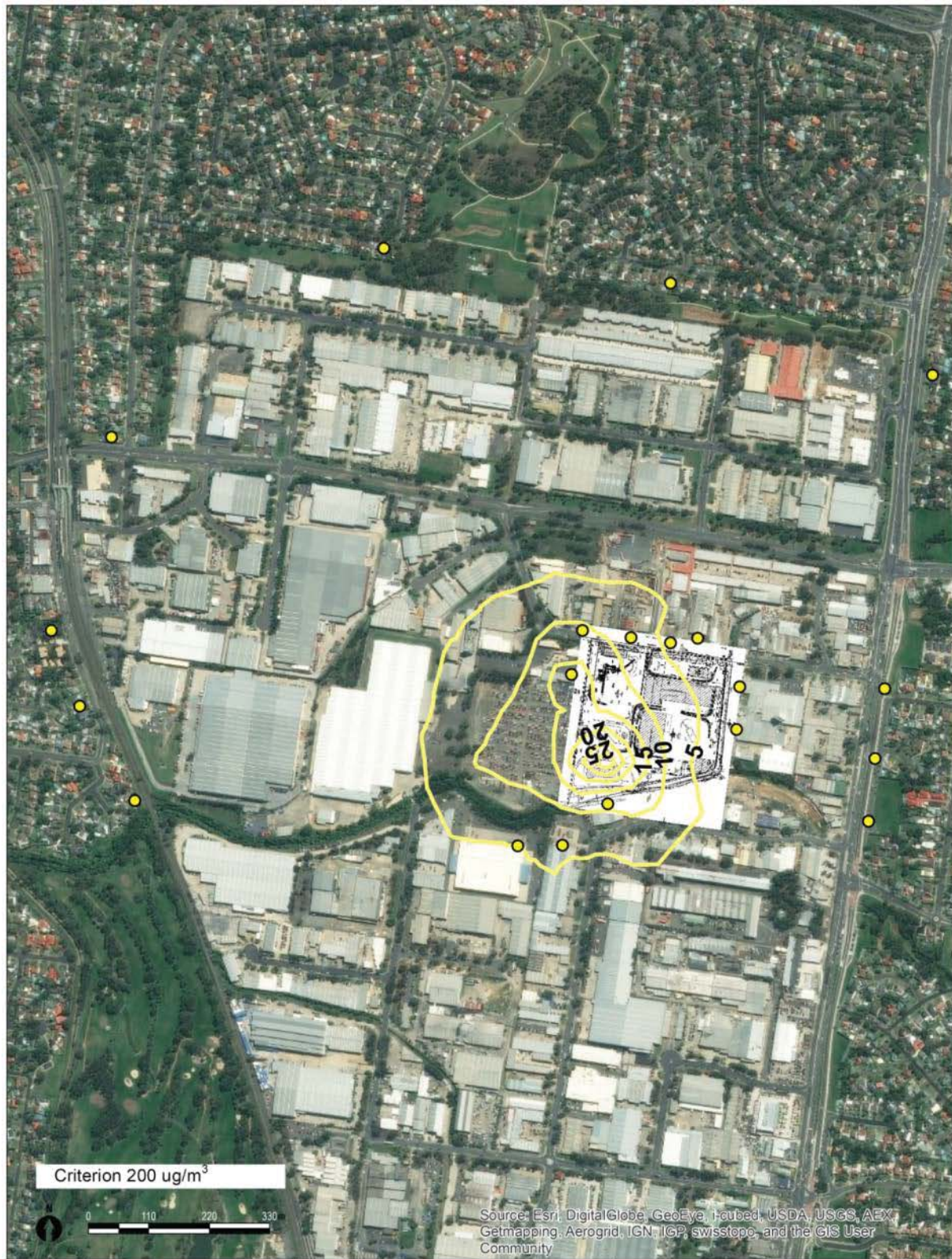
Figure B.23 Maximum (99.9 th percentile) predicted (over five years) Site contribution to 8-hour average (TWA) copper dusts and mists concentrations (excluding background) with cutting modelled as point sources
