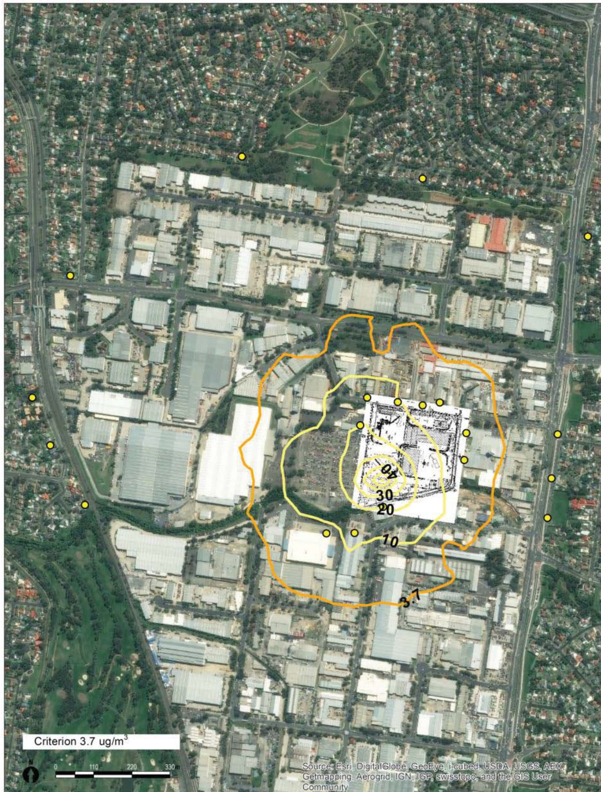
Figure B.22 Maximum (99.9 th percentile) predicted (over five years) Site contribution to hourly copper dusts and mists concentrations (excluding background) with cutting modelled as point sources
