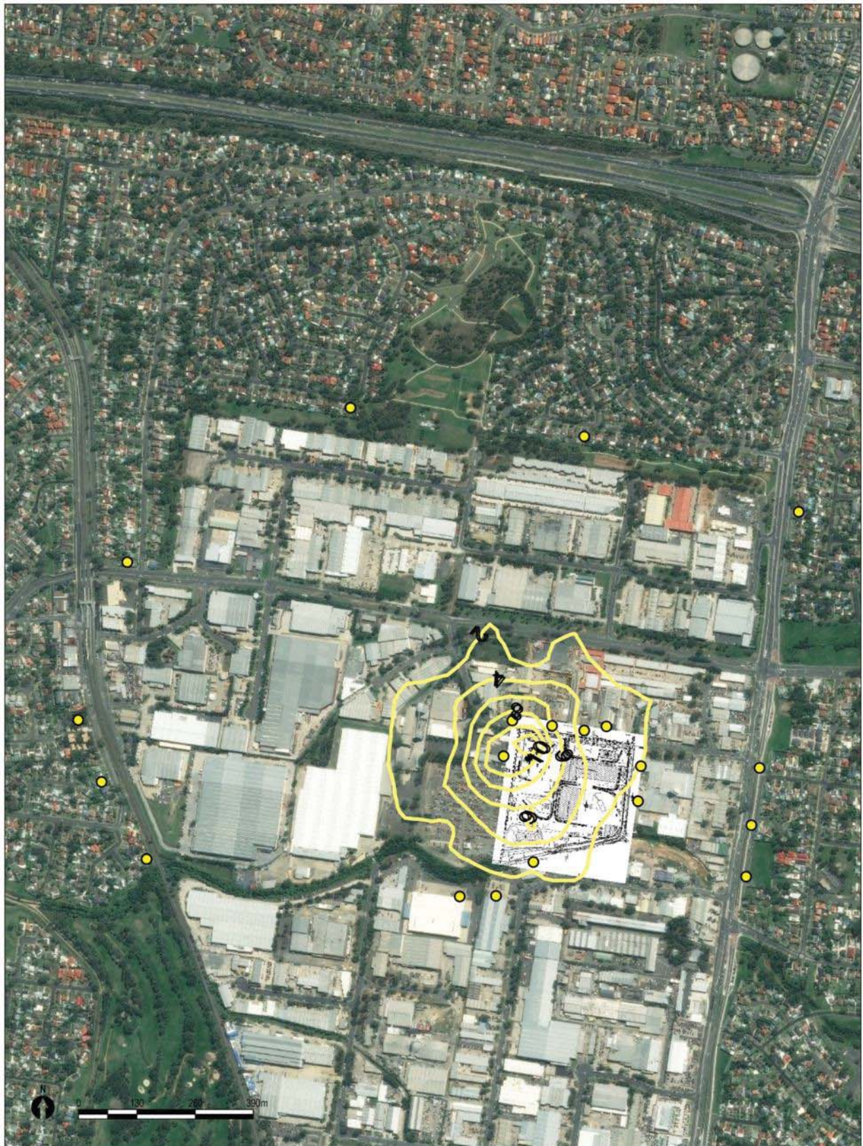
Figure B.1 Maximum predicted (over 5 years) Site contribution to annual average TSP Concentrations (excluding background)
