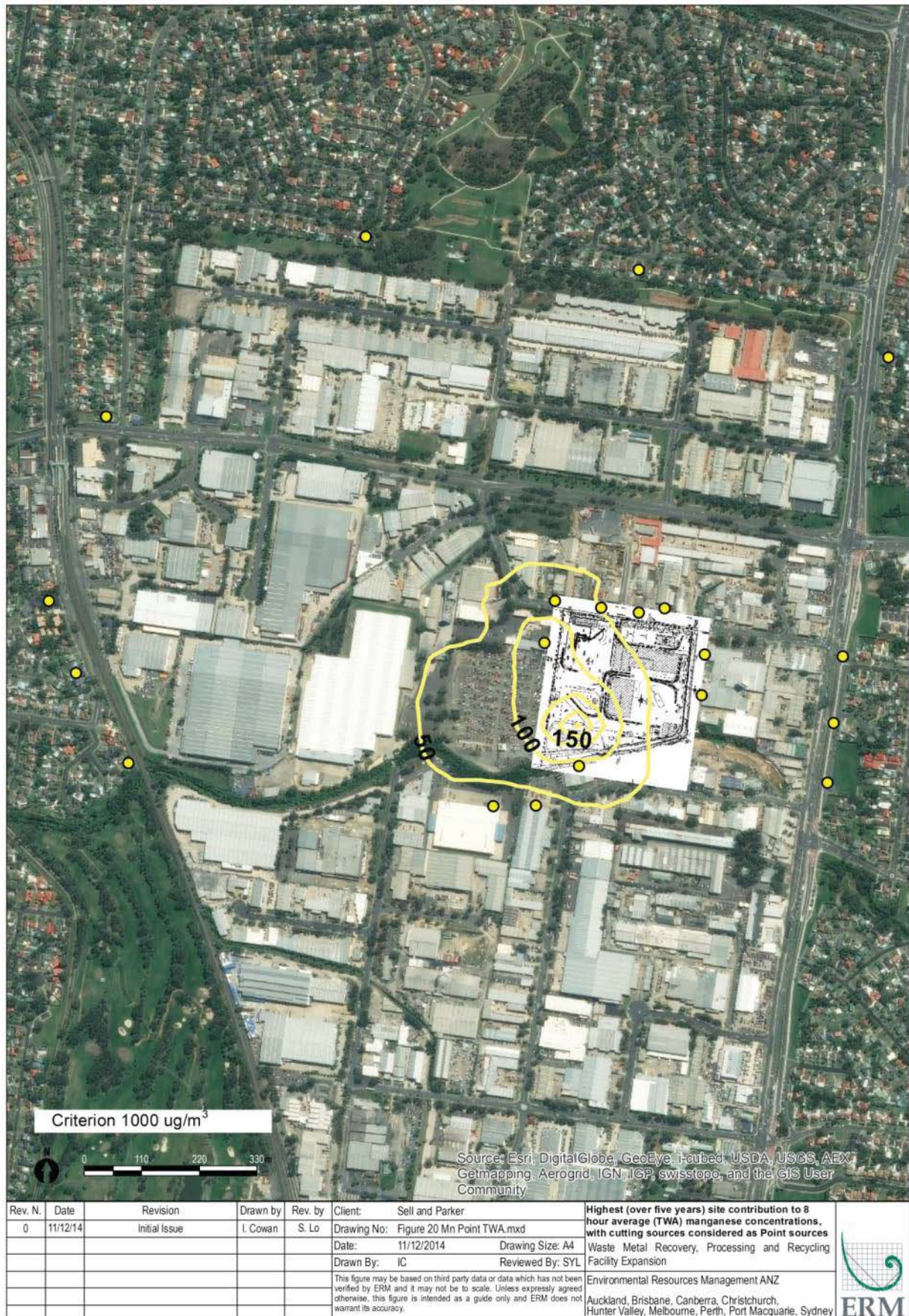
Figure B.20 Maximum (99.9 th percentile) predicted (over five years) Site contribution to 8-hour average (TWA) manganese and compounds concentrations (excluding background) with cutting modelled as point sources
