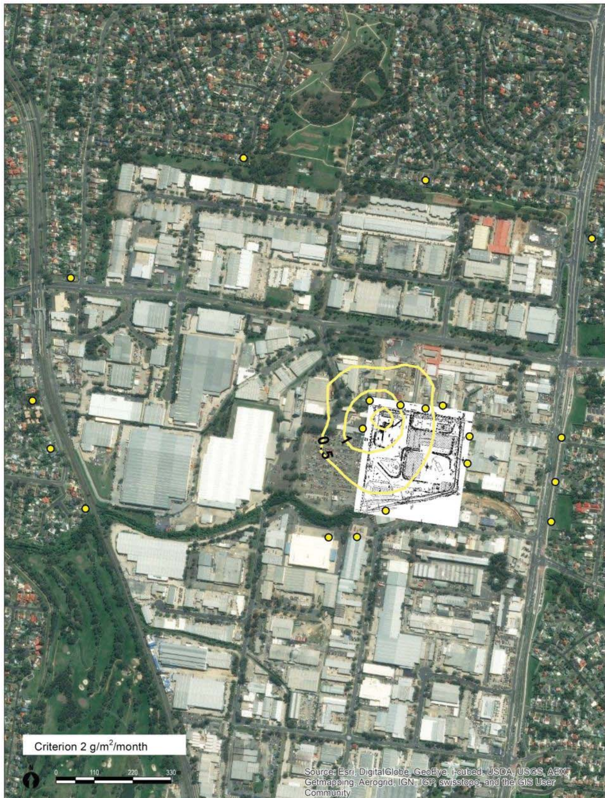
Figure B.2 Maximum predicted (over 5 years) Site contribution to annual mean Dust Deposition (excluding background)
