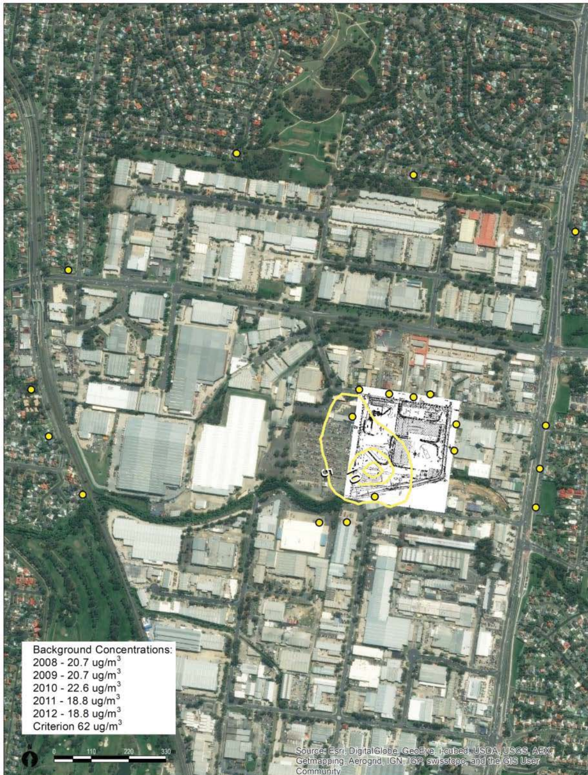
Figure B.10 Maximum predicted (over five years) Site contribution to annual average NO 2 concentrations (excluding background) with cutting modelled as volume sources
