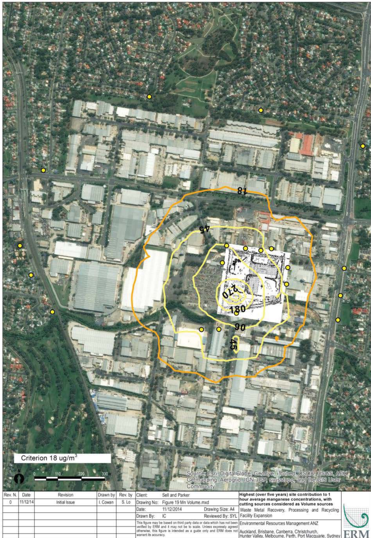
Figure B.18 Maximum (99.9 th percentile) predicted (over five years) Site contribution to hourly manganese and compounds concentrations (excluding background) with cutting modelled as volume sources
